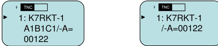
Above is an example of the Kenwood TH-D7 screen with telemetry bits A, B, and C enabled. The GPS is not locked, and the altitude is 122 meters. All of the input bits are pulled high. To the right is the display with the digital telemetry bits disabled.
