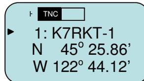
Above is an example of the Kenwood TH-D7 screen showing the latitude and longitude display of an APRS formatted packet. TEXT formatted packets can be decoded by other devices including the PicPac from Byonics.
