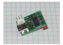
The BigRedBee USB interface integrates the functionality of two separate devices; a USB data interface, and a single cell lithium poly battery charger.
